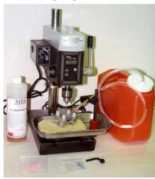
NOTE: THIS SYSTEM IS DESIGNED FOR A DRILLING A MAXIMUM OF 1/4" Dia. HOLES
