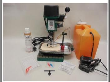
NOTE: THIS SYSTEM IS DESIGNED FOR A DRILLING A MAXIMUM OF 1/4" Dia. HOLES
